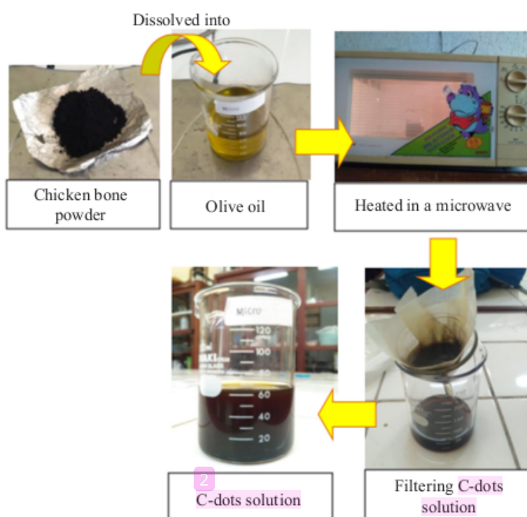
Figure 2: The C-dots synthesis procedure.
